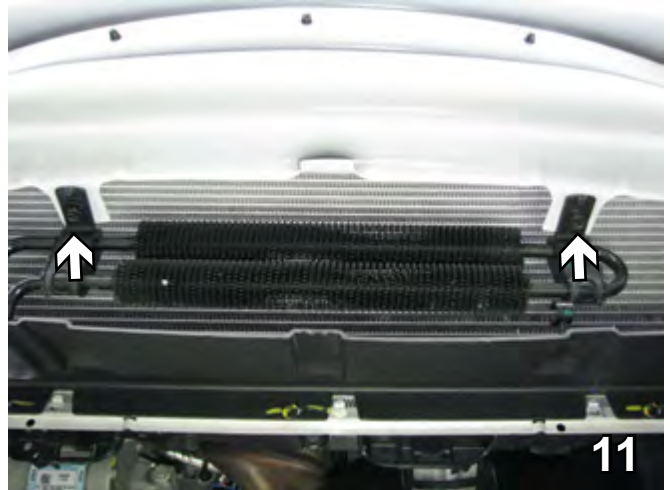
11. Unbolt the coolant line and set it down, out of the way.
