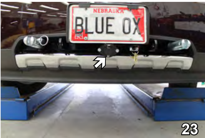
23. Reinstall the fascia. Attach the electrical bracket to the center of the fascia.
