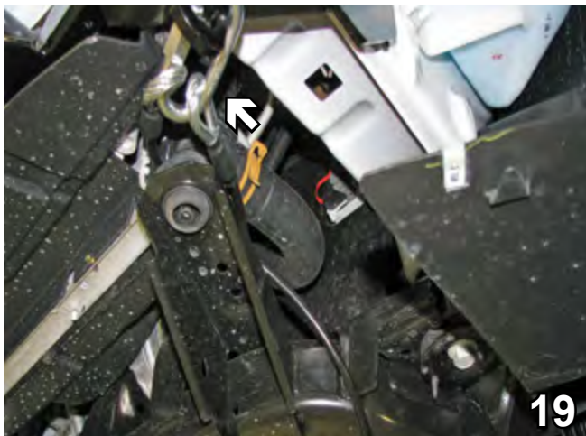
19. Attach the permanent baseplate safety cables to the provided convenience link on the baseplate (see white arrow). The photo above shows the recommended installation of the cables to frame of vehicle. Additional options may interfere with suggested mounting; in this case secure the cables to a solid piece of the frame as described in the instructions included with the permanent baseplate safety cables. Be sure the safety cables do not rub against any hoses or moving parts. Do this to both sides of the vehicle.
