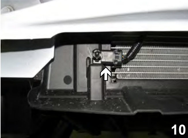
10. On the passenger side behind the bumper, move the temperature sensor and zip tie it.
